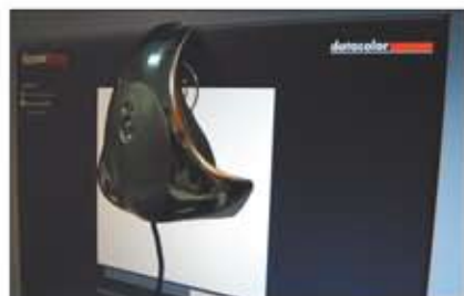
The colorimeter mounted via its suction cup on the LCD screen. This new sensor packs an improved sensitivity over its antecedent.
